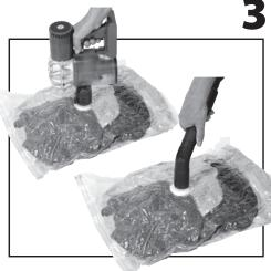
Note: Some vacuum connectors may not fully cover the valve seal. To speed up suction, cup one finger around the nozzle. Alternatively, wrap the nozzle in either sticky tape, electrical tape, aluminum foil or cling wrap if necessary.
